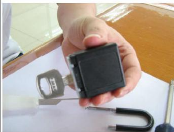
13. dress the plastic jacket on alum body
