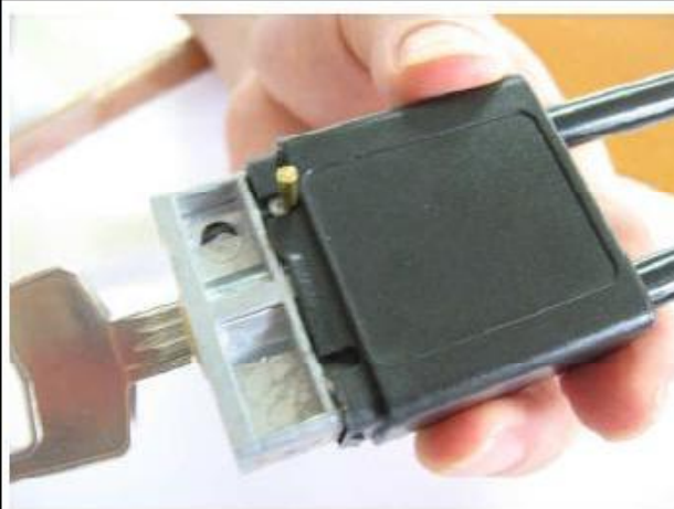
15. press in the shackle retaining pin
