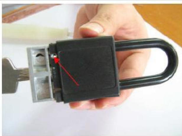
14. assemble shackle and push the body out from the jacket until the shackle retaining holes on alum body and plastic jacket overlapping
